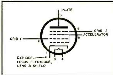
Fig. 3. Schematic symbol of the 6BN6 tube.
