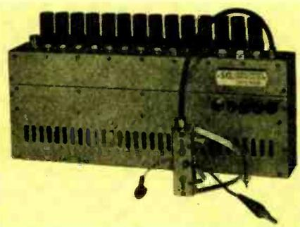
passband, and the power supply is stabilized to prevent fluctuations of gain due to variations in the signal duty factor. For further information, write to *Spencer-Kennedy Laboratories, Inc.*, Dept. RT, 186 Massachusetts Avenue, Cambridge 39, Mass.
