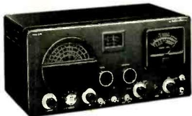
**Top Selectivity—Low Price! Model S76**—Dual Conversion Super with 50 kc amplifier for tops in selectivity, 500 C.P.S. at 6 db down—3.5 kc at 60 db down. Giant 4-in. "S" meter. 540-1580 kc, 1.72-32 Mc in 4 bands. 1 r-f, 2 conversion, 2 i-f stages. 5 pos. selectivity. Phono input jack. 3 watt output. **\$179.50**
