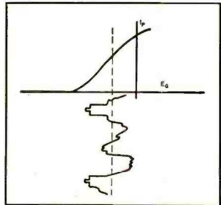
Fig. 4. The first video amplifier of Fig. 1 is operating over most of its range with normal signals; negative noise pulses are cut off.
