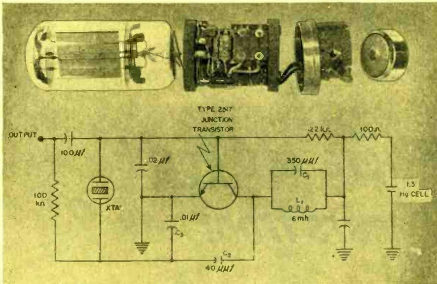
Exploded view and circuit diagram of the NBS transistor oscillator.
