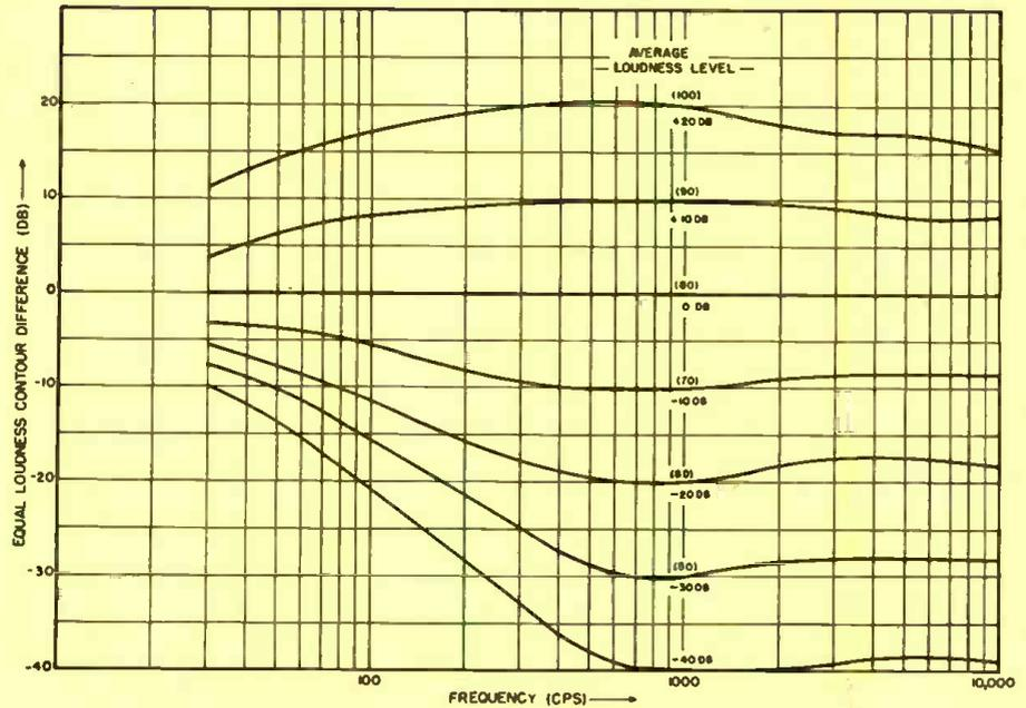
Fig. 2. Difference contours referred to 80 db as a basic level.
