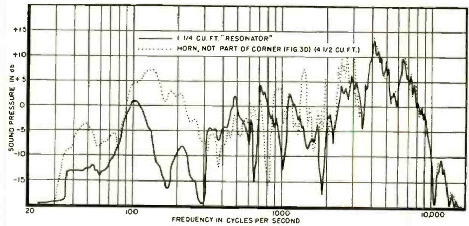
Fig. 10. Relative response of a  $1\frac{1}{4}$  cu. ft. resonator and a  $4\frac{1}{2}$  cu. ft. horn which is not part of the corner. See the test set-up shown in (D) of Fig. 3.
