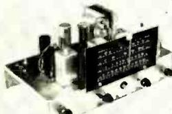
Three Band Model AR-1 6 Tube all wave circuit 3 Ranges, continuous coverage 550 KC to over 20 MC. Shipping Weight 11 lbs.
