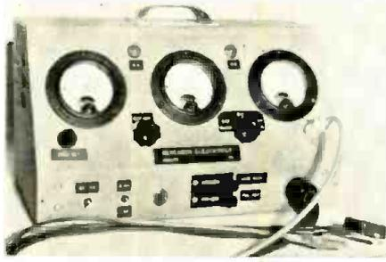
tive), grid-cathode leakage, A2 leakage, and G2 leakage. It features electronically-controlled and regulated circuits. The unit operates from 117 volt, 60 cycle a.c. lines.
