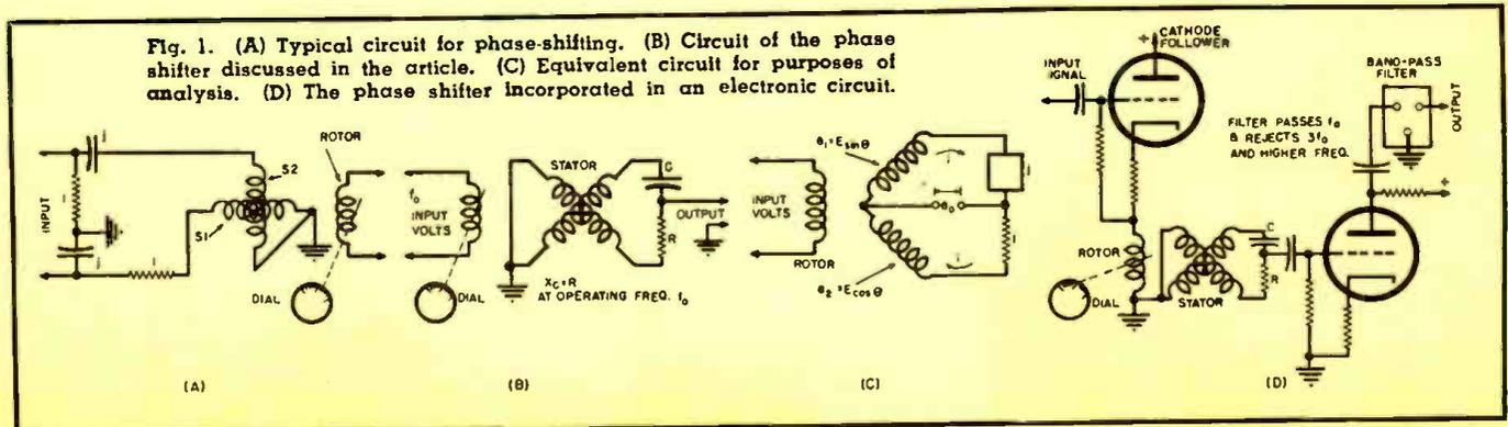
Fig. 1. (A) Typical circuit for phase-shifting. (B) Circuit of the phase shifter discussed in the article. (C) Equivalent circuit for purposes of analysis. (D) The phase shifter incorporated in an electronic circuit.
