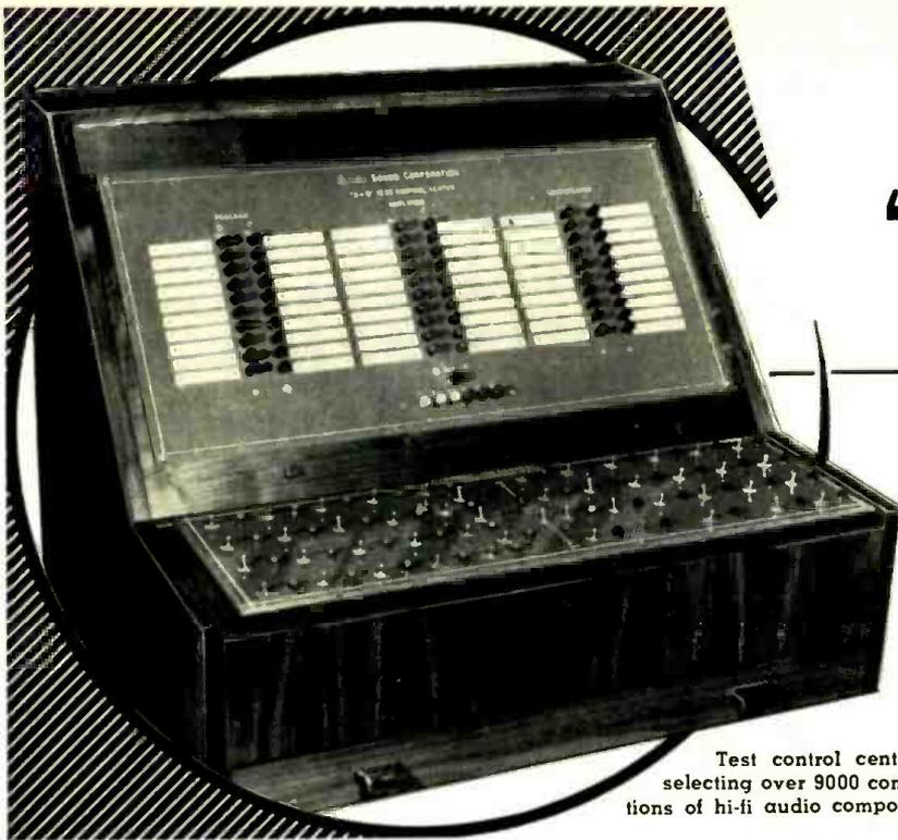
Test control center for selecting over 9000 combinations of hi-fi audio components.
