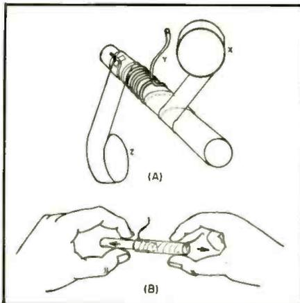
Fig. 1. (A) Steps in preparing rod and winding coil. (B) How coil is removed from rod.
