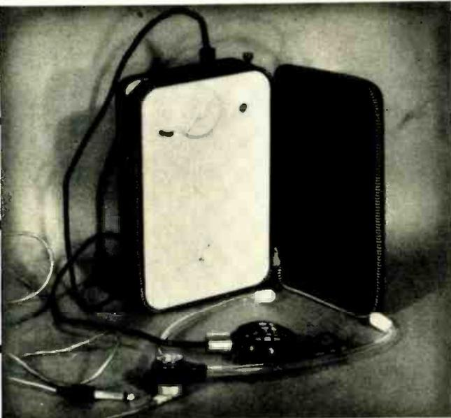
Fig. 1. The "Minifon" measures but  $4\frac{5}{8}$ " x 7" x 2" when contained in its soft leather zipper case. Crystal diaphragm microphone and stethoscope-type earphones come with each recorder.
