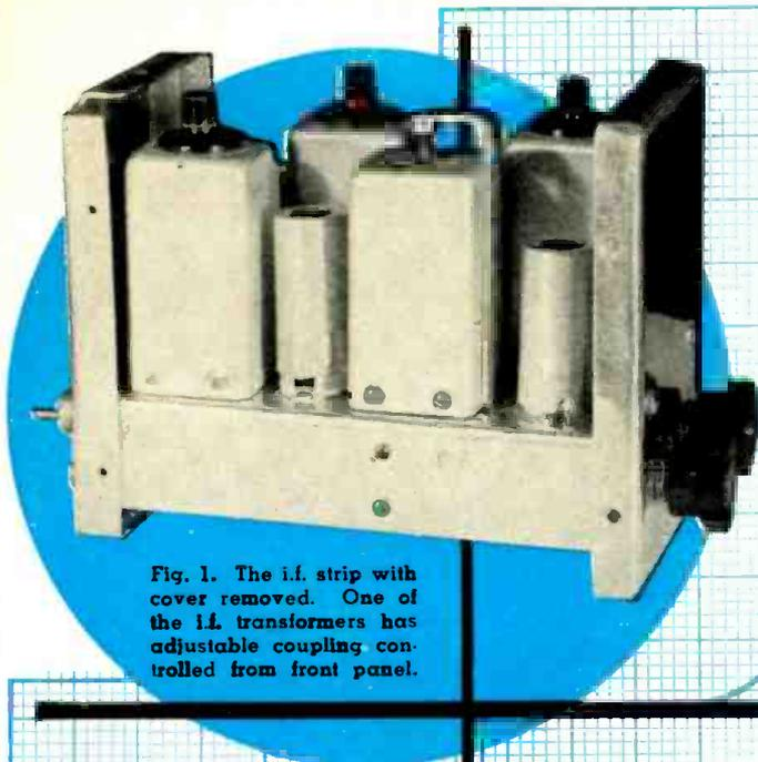
Fig. 1. The i.f. strip with cover removed. One of the i.f. transformers has adjustable coupling controlled from front panel.
