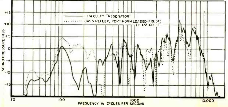
Fig. 12. Relative response of the  $1\frac{1}{4}$  cu. ft. resonator and a  $4\frac{1}{2}$  cu. ft. bass reflex with the port horn loaded as illustrated in the diagram of Fig. 3F.
