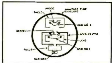
Fig. 5. Internal construction of the 6BN6.
