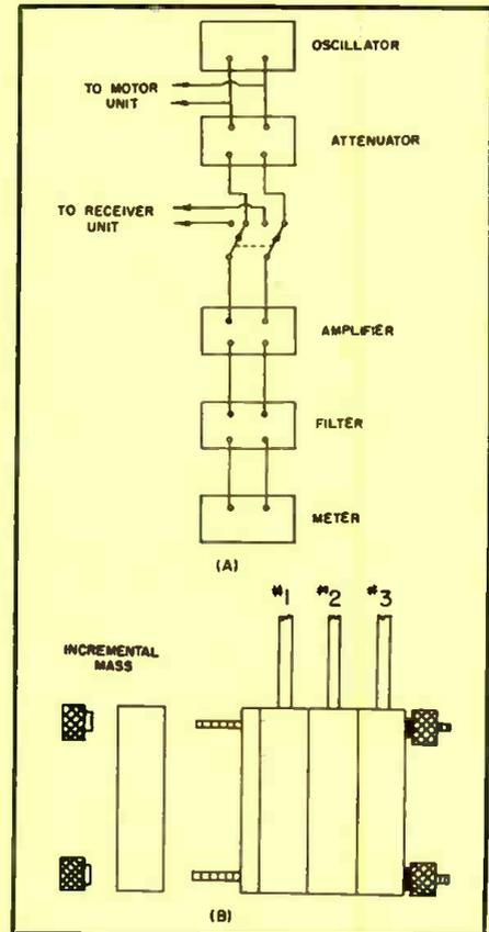
Fig. 2. Calibration of vibration pickups by the reciprocity method.
