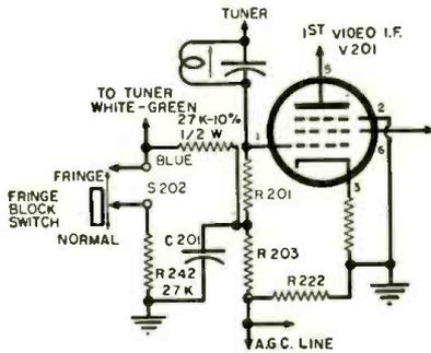
sistor between the junction of R201-R203 and the junction of the blue and white-green leads.
