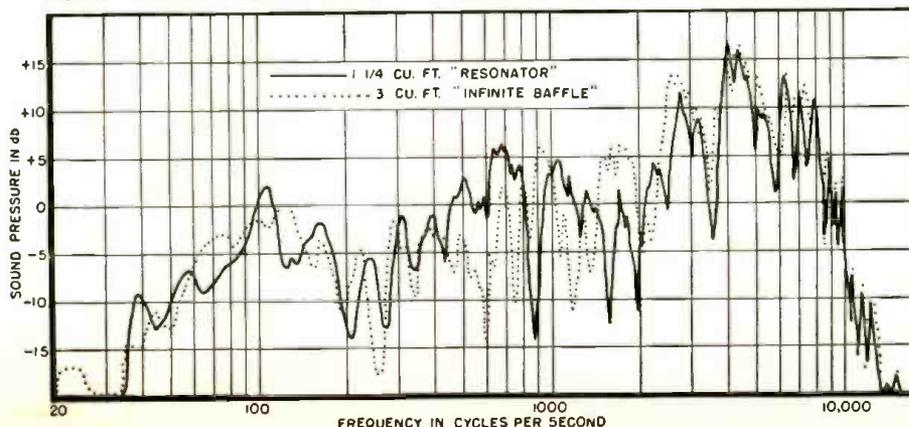
air resonance of the speaker. The general effect of the infinite type of baffle with no acoustic compensation is to tighten up the speaker in a limited frequency range.
