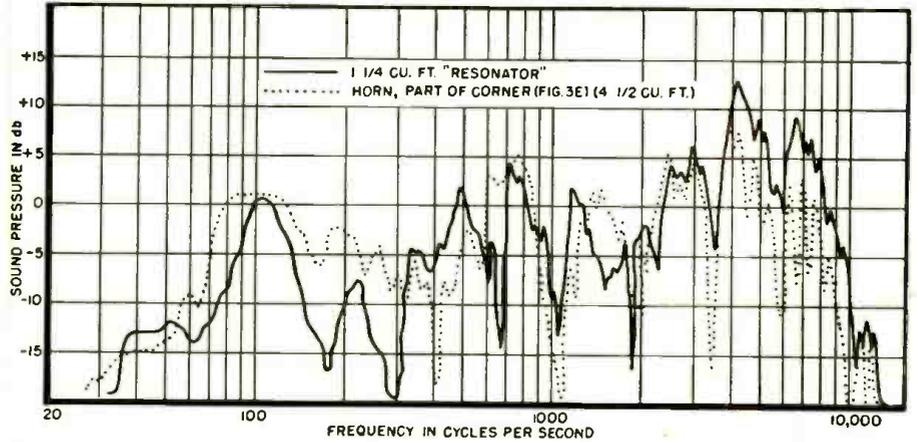
Fig. 11. Relative response of the  $1\frac{1}{4}$  cu. ft. resonator and a  $4\frac{1}{2}$  cu. ft. horn which is a part of the corner of the test room. Refer to Fig. 3E for details.
