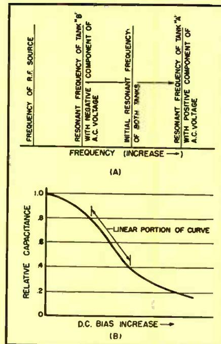
Fig. 4. (A) Tank circuit relationships of Fig. 5B. (B) Capacitance vs. d.c. bias curve for  $K=3300$  dielectric material.
