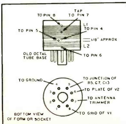
Mechanical details and winding data on coils  $L_1$  and  $L_2$  for the regenerator.
