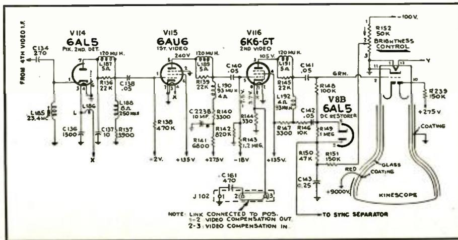
current, but only if it is strongly negative. If it is made zero or positive, it will permit electrons to pass without altering their number. In other words it functions as an open gate, while grid #1 determines the extent of the tube current flow.
