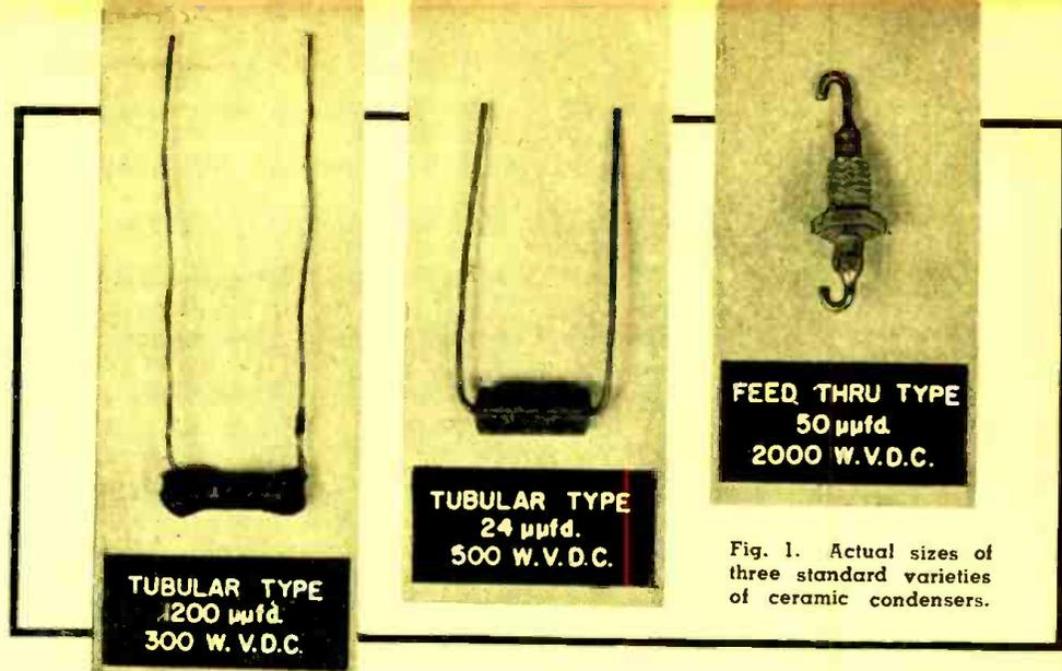
Fig. 1. Actual sizes of three standard varieties of ceramic condensers.
