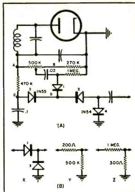
Fig. 2. (A) The full-wave compound limiter. (B) Attenuation network: basic circuit, X; signal conditions, Y; noise conditions, Z.
