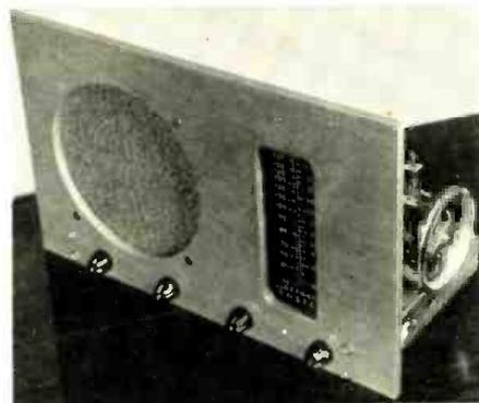
transformer, the set, known as the Model R-1 chassis, gives 5 watts' output. It is equipped with a phono jack and a phono position on the band-switch for use with a record changer or player.
