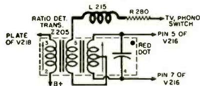
for the presence of L215, fixed inductor, connected between pin 5 of the ratio detector transformer, Z205, and one end of resistor R280 (270 ohm, 1/2 w. carbon). If L215 is present, remove it and connect R280 directly to pin 5 of Z205.
