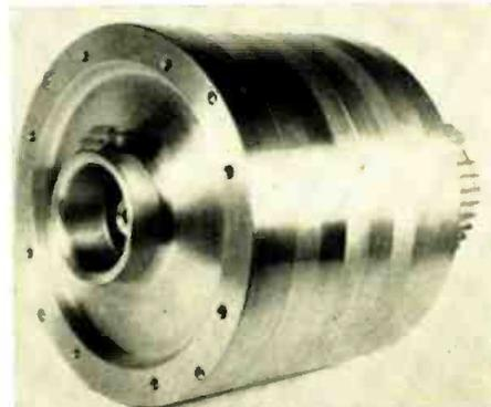
high air pressures are required in combination with relatively low volumes, these new units are powered by totally enclosed induction motors built on a single shaft with the blower.
