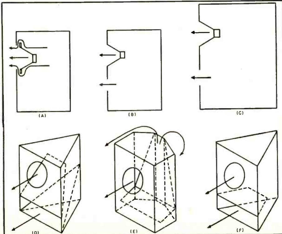
is a pure transmission line terminating at one end in the speaker impedance and at the other end into the characteristic acoustic impedance of open "space." If properly designed, such a transmission line acts as an untuned device, or "anti-resonant." In addition to being anti-resonant in themselves, horns serve to damp out speaker resonances by loading the speaker with an acoustic column of air before its radiation hits free space. An increase in low frequency efficiency is the usual result.
