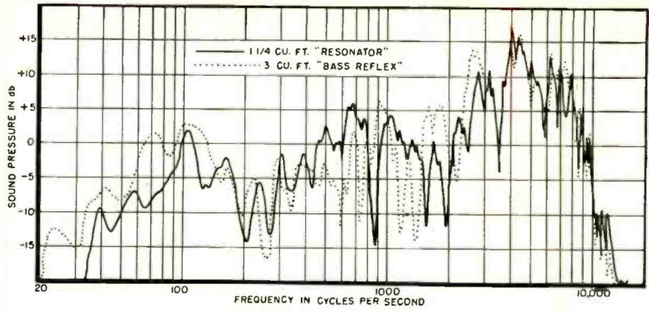
Fig. 9. Relative response of a  $1\frac{1}{4}$  cu. ft. resonator and a 3 cu. ft. bass reflex.
