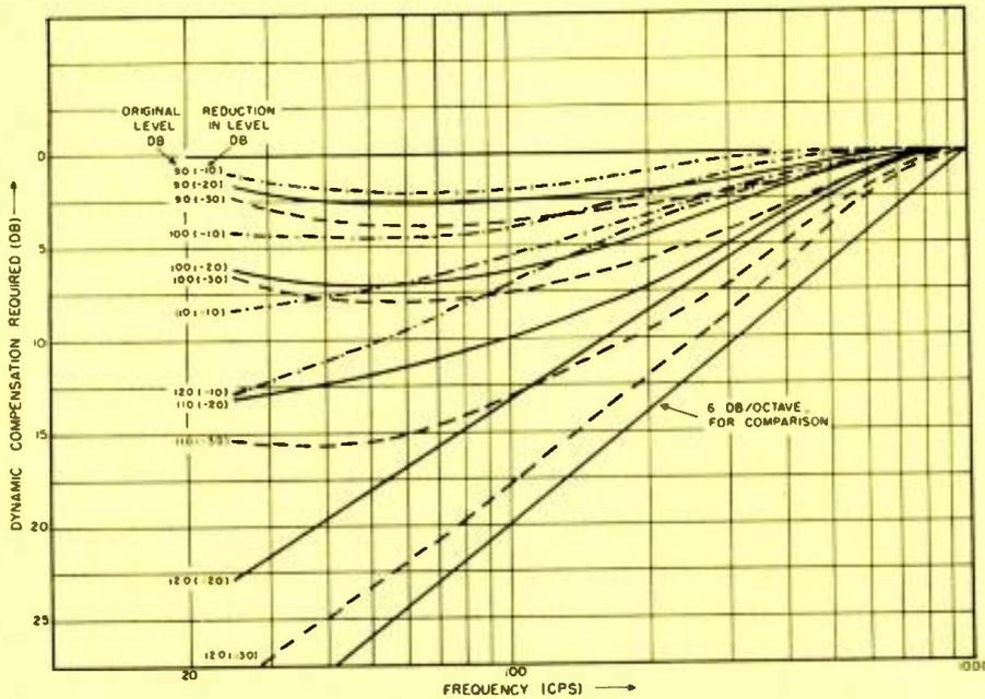
Fig. 4. Dynamic compensation required in addition to that afforded by the so-called static type of loudness control.
