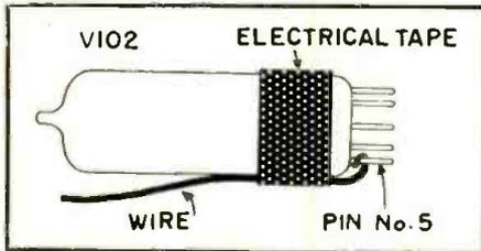
Fig. 8. A convenient method for applying alignment signal to mixer-oscillator.
