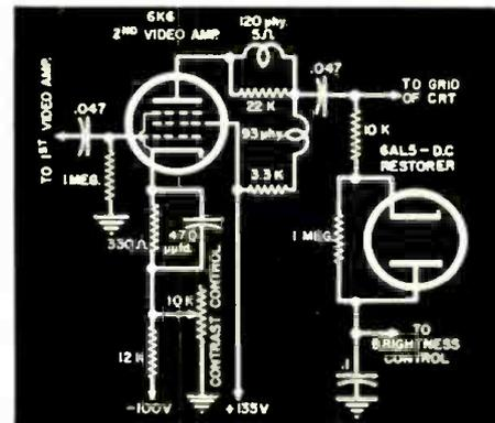
Fig. 2. Contrast control circuit which leaves sync pulse unaffected during adjustment.
