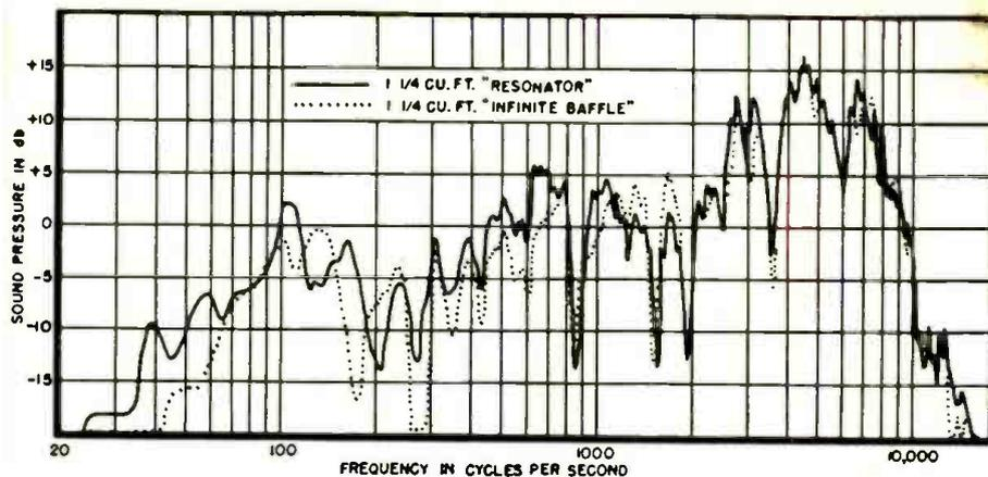
Fig. 4. Relative response of the Helmholtz resonator and an infinite baffle type.
