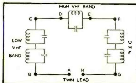
the appropriate choice of "Q" and L/C ratio for each network, it is possible to connect the v.h.f. and u.h.f. antennas simultaneously to a single pair of downleads, and have each properly terminated in the 300-ohm receiver input (over its appropriate frequency range) with a minimum insertion loss and voltage standing wave ratio.
