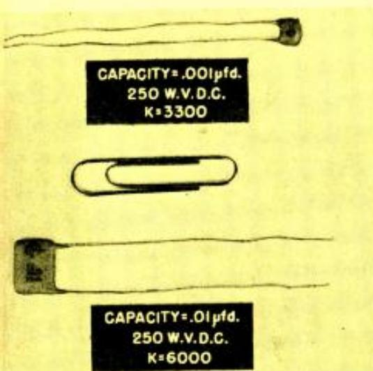
Fig. 2. Two very high K nonlinear condensers are shown in their actual sizes.
