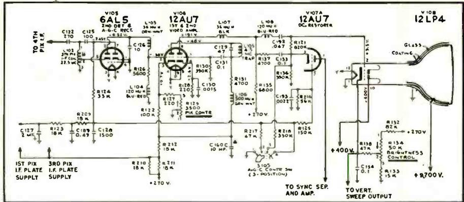
Fig. 2. Improved version of noise suppression circuit shown in Fig. 1.
