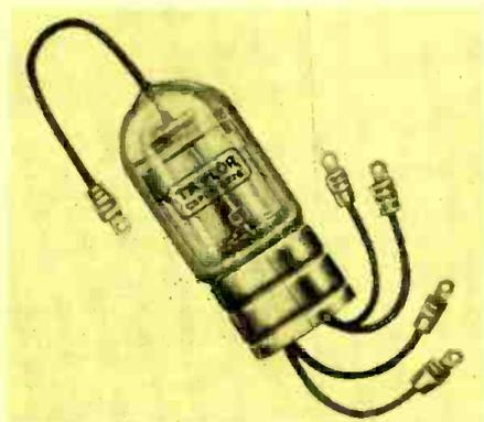
medium cap without flexible lead. Average anode current is 3 amp., peak anode current 30 amp., peak anode voltage 1000 volts. Deionization time is under 175 microseconds.
