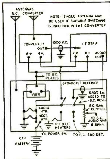
Fig. 6. External connection diagram. Most of the car receiver is disabled to save power when the attached equipment is used.
