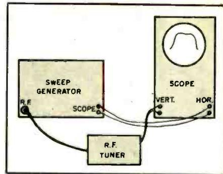
Fig. 2. Test setup for visual alignment.
