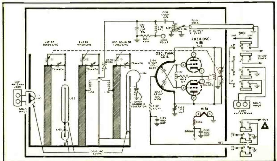
Fig. 2. Complete schematic diagram of the Du Mont RA-166/167, 170/171 chassis.
