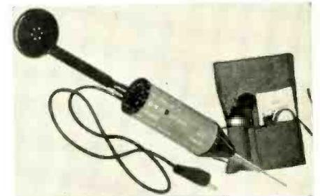
a.g.c. and a.v.c. resistors; substitution and test for medium value dropping, plate load resistors, etc.; substitution and test for low value cathode bias, current limiting resistors, filter chokes, etc.; and a dynamic checker for speakers, phones, etc.
