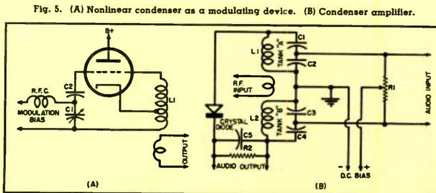
Fig. 5. (A) Nonlinear condenser as a modulating device. (B) Condenser amplifier.
