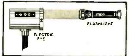
Fig. 4. Test set-up for photocell relay.
