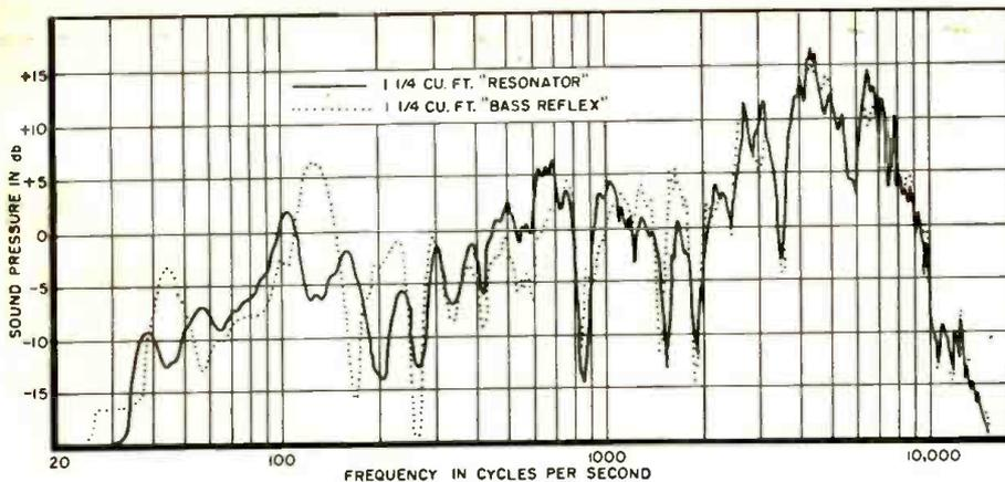
Fig. 6. Relative response of a 1/4 cubic foot resonator and bass reflex of same size.
