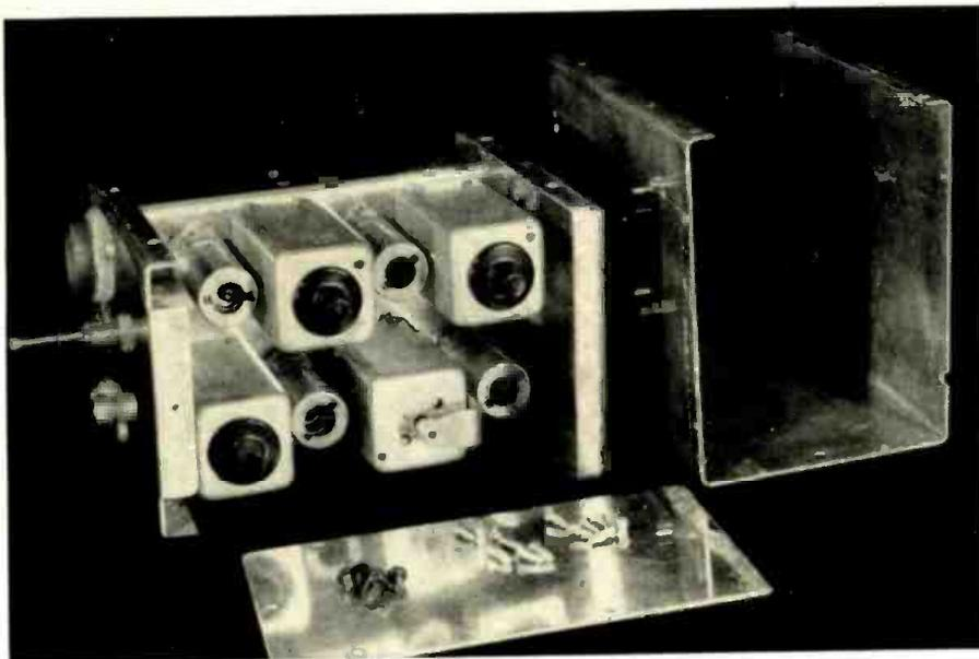
Fig. 3. Top view, showing tube and transformer layout and sheet-metal covers. The method of adjusting the coupling of  $T_1$  (lower right) is explained in the text.
