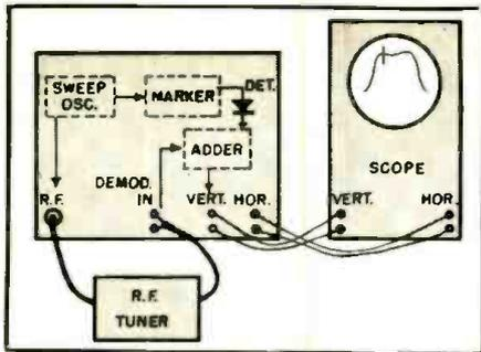
Fig. 4. Visual alignment setup using u.h.f. sweep generator which adds marker to detected sweep signal after it comes from tuner.
