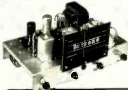
Broadcast Model BR-1 5 Tube Broadcast Band 550 to 1600 KC coverage. Shipping Weight 11 lbs.
