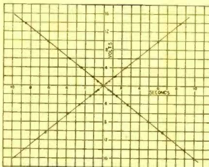
Fig. 9. Graph showing the response of an integrator to a step input.
