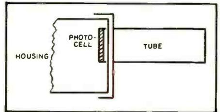
Fig. 3. A shield in front of cell cuts off light which might strike cell from an angle. Suitable for door-opener application.
