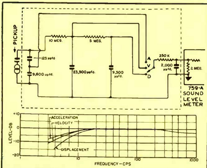
Fig. 4. Inertia-type pickup and approximate equivalent circuit.
