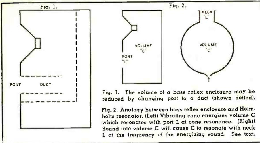
Fig. 1. The volume of a bass reflex enclosure may be reduced by changing port to a duct (shown dotted).
