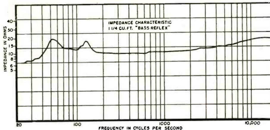
Fig. 7. Impedance characteristic of the 1/4 cubic foot bass reflex type cabinet.
