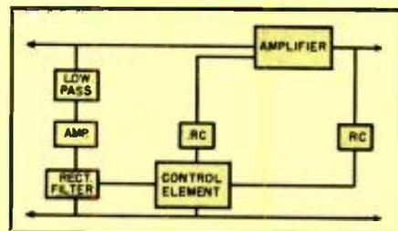
Fig. 6. Block diagram for negative feedback dynamic loudness control.
